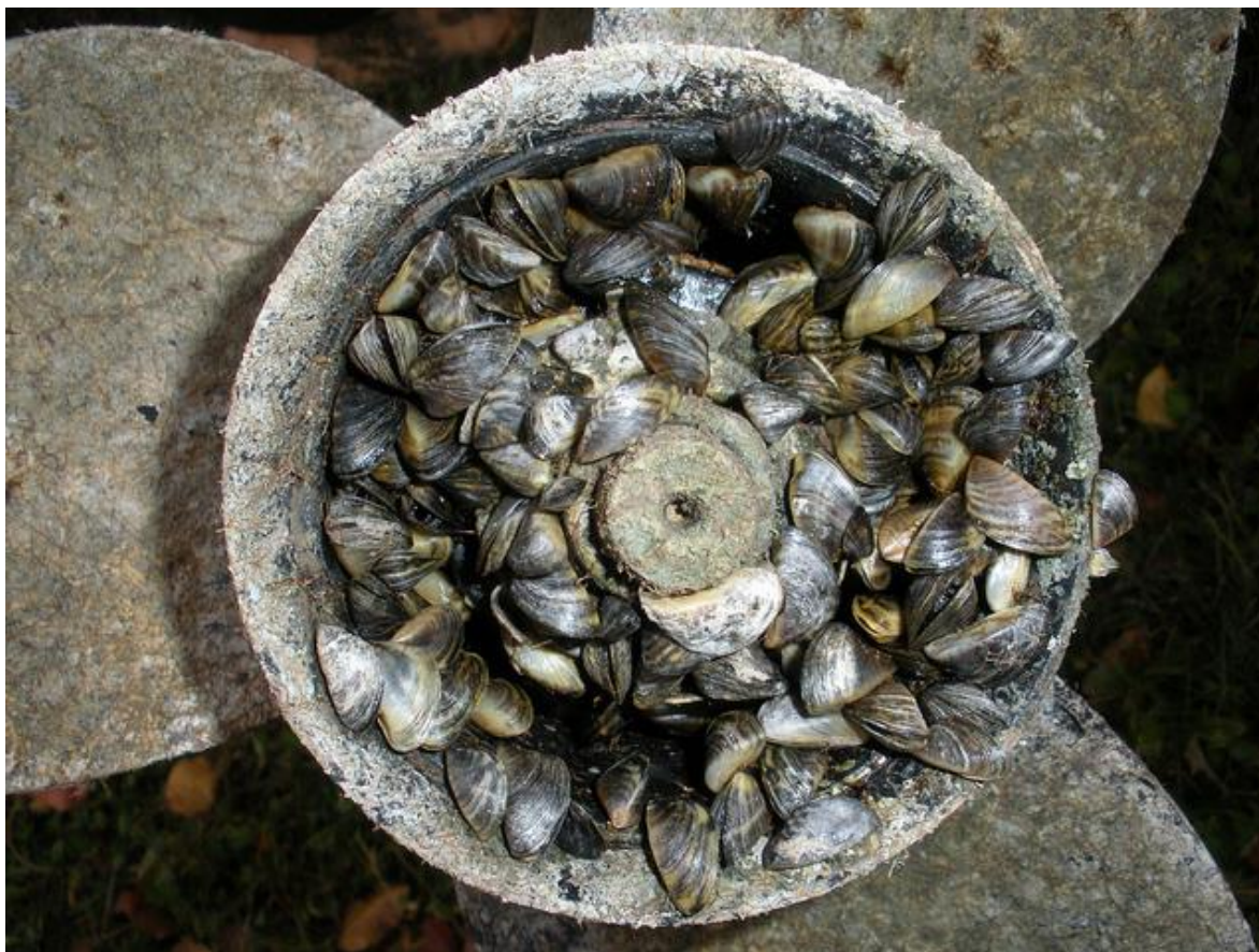
Figura 29. Turbina infestada por mejillones cebra. Tomado de https://www.google.com/url?sa=i&source=images&cd=&ved=2ahUKEwik9N3BhdPjAhUKUK0KHWRLBucQjRx6BAgBEAU&url=https%3A%2F%2Fstateimpact.npr.org%2Ftexas%2F2013%2F06%2F18%2Fhow-zebra-mussels-could-raise-your-water-bill%2F&psig=AOvVaw23KmtN85PLT7vylEAeT1iV&ust=1564246239801469
